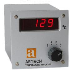
The Artech Multipoint Digital Temperature Indicator Model 200M provides an accurate indication of temperature with a resolution upto 0.1°C. The fully solid state circuitry with no plug-in cards enables the instrument to withstand severe vibrations and shocks. Thermocouple break indication, automatic lead resistance compensation and automatic cold junction compensation are added features of this instrument.
