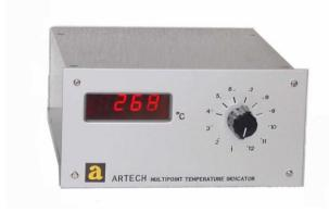
Multipoint Digital Temperature Indicator Model 230M provides an accurate indication of temperature with a resolution upto 0.1°C. The fully solid state circuitry with no plug-in cards enables the instrument to withstand severe vibrations and shocks. Thermocouple break indication, automatic lead resistance compensation and automatic cold junction compensation are added features of this instrument.
