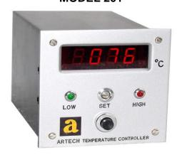
The Artech Temperature Controller, Model-201 is a compact, sturdy instrument useful for furnaces, ovens, processing industries and laboratories. Sensor break protection and ambient compensation are standard features. Set point selection is by means of a single ten turn Potentiometer. Depressing the `SET' switch displays the set point. In normal operation the display indicates actual temperature.
